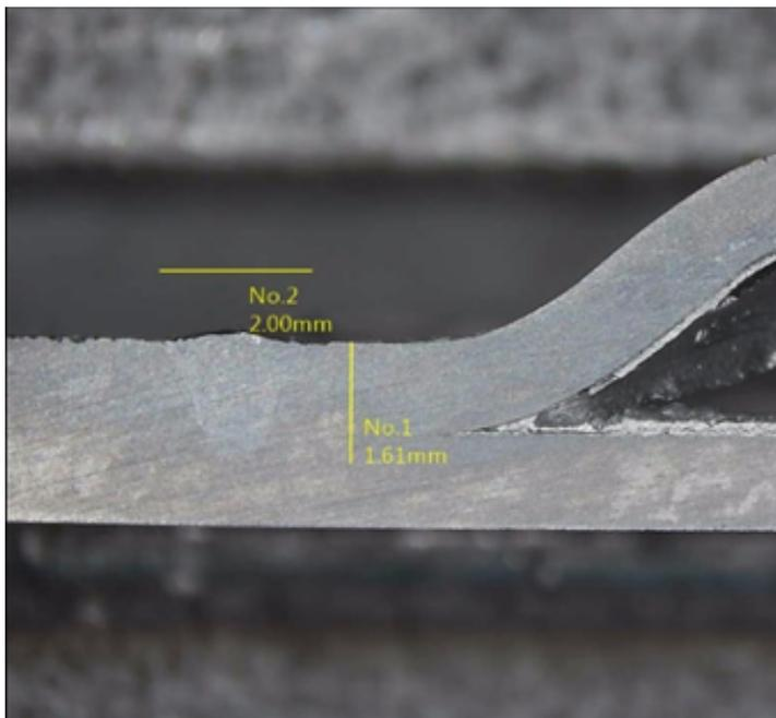
**In these materials, DBL technology can achieve stable welding of cooling plate seams at feed rates of 30 m/min. The DBL achieved 30-meter-long weld seams with consistent geometry on each plate.**
