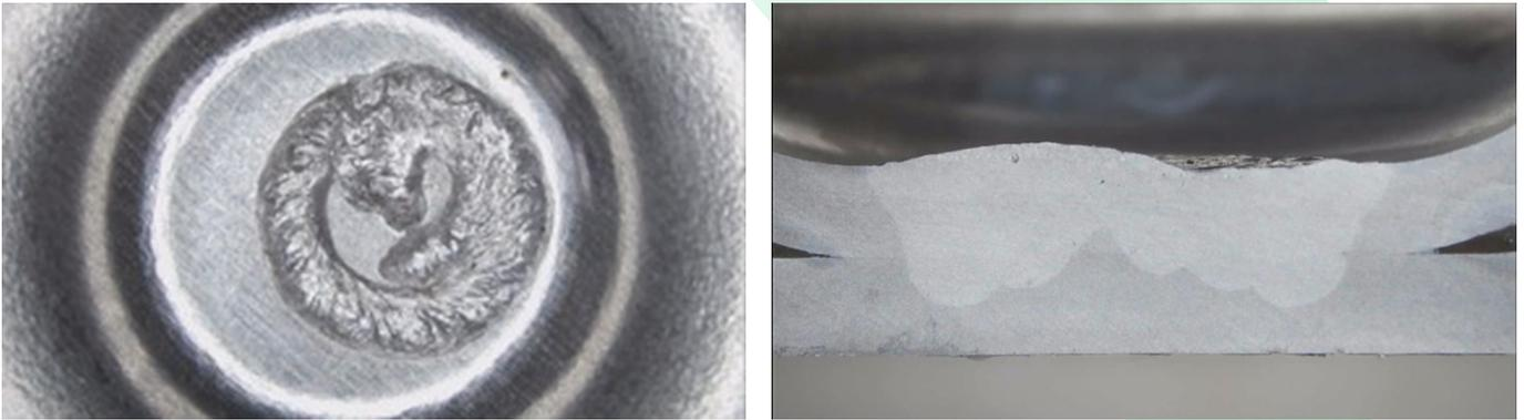
**Figure 4:** Some designs included large area welds, which caused hot cracks. By using complex beam shapes, DBL technology was able to prevent these defects.
