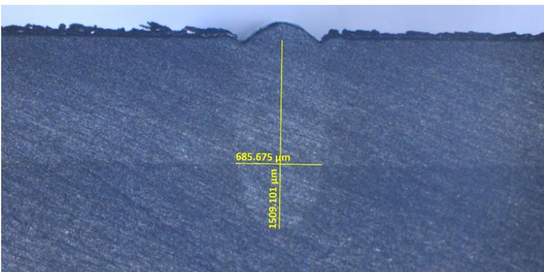
**Figure 5:** Another design included asymmetrical material, with the top plate measuring 1 millimeter in thickness and the bottom plate measuring 3 millimeters.
