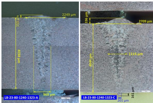
Fig. 5. Microsections of the copper butt-welds, 10  $\mu$ s per shape.
